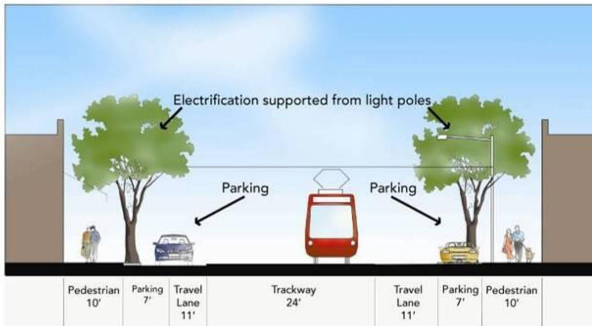
**Figure 4.** Santa Monica design for LRT in Colorado Avenue, with 80-foot/24.2-m ROW. (Graphic: City of Santa Monica)
