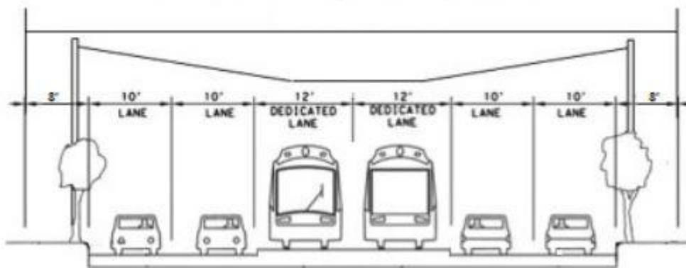
**Figure 6.** LRT alignment cross-section design for Austin's Guadalupe-Lamar corridor. (Graphic: Author)
